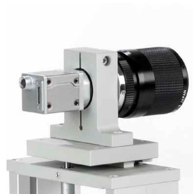
LMO 0103 Telecentric lens of the LSA 100 Research
