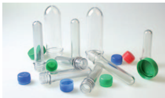
Preforms for creating PET bottles. The IV value needs to be at least 70 cm 3 /g.
